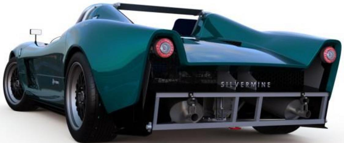
At the rear, the exposed chassis frame shows its raw engineering and functionality. Underneath the tailgate, the engine bay is visible as is the gear lever mechanism and the adjustable rear suspension. The complete exhaust system is not even styled at all.
