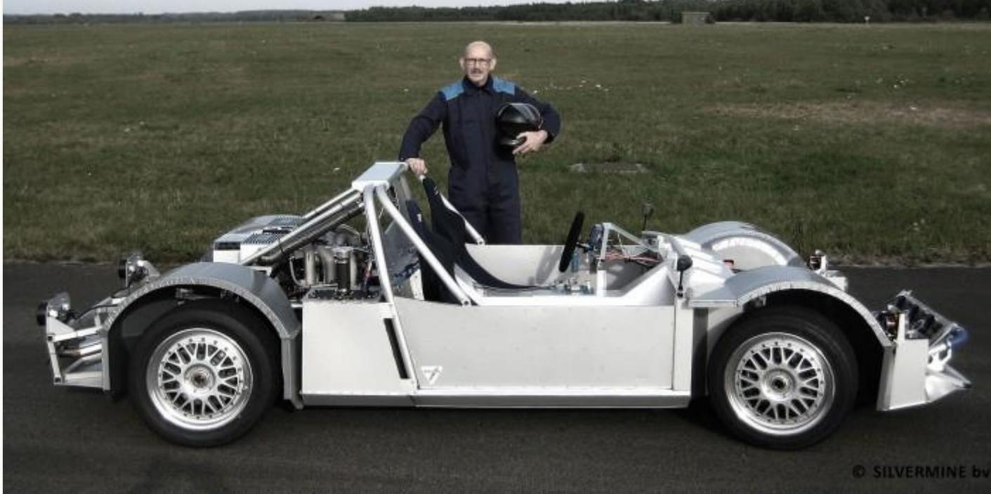
The car features an aluminum space frame chassis and is equipped with a 325hp 6-cylinder Subaru boxer engine, coupled with a six-speed sequential gearbox and a limited slip differential.
