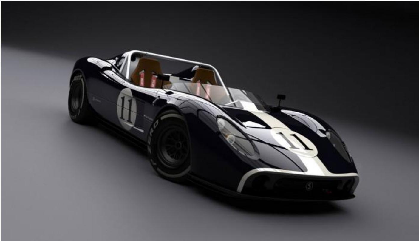
The air ducts are kept simple and purely functional, no excessive design is applied. The form language of some elements are inspired by elementary fabrication techniques, like the front nose grill (milling aluminium), side skirts and rear diffuser (pressing and bending sheet metal).
