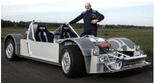
The project in question is called the Silvermine 11SR. It's the brainchild of Frank van Rouendal, a marine engineer and machine constructor based in Overdinkel, Holland. Designed by brothers Marco and Andries van Overbeeke, the Silvermine 11SR is being built around an F1-style safety cell with a Subaru-sourced 3.0-liter boxer six that develops 325 horsepower.
